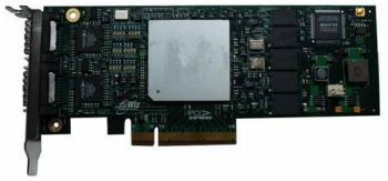
2-port, 10 Gigabit Ethernet PCI-Express NIC TCP/UDP/IP acceleration IPv4 and IPv6 copper/fiber optic
