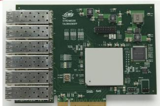
Regeneration Ethernet TAP Card Optic/Copper Media Converter Packet Filter, Line monitor
