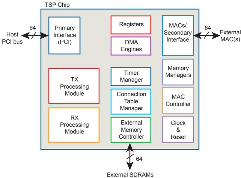
TCP/IP Offload Engine Chip LE2020™
