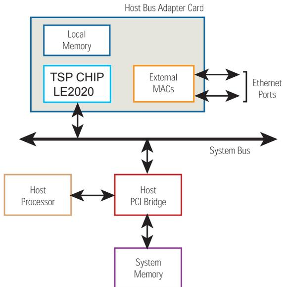
Dual Gigabit HBA Card with LE2020™ TCP/IP Offload Engine
